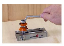
Unscrew the top nut with an appropriately sized wrench to disassemble the router bit.
