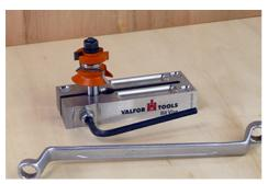
Once the Bit Vise is securely fastened, the router bit can be inserted into the appropriate hole. Using the supplied hex key, turn the bolt clockwise to tighten the jaws of the Bit Vise around the router bit's shank just enough to avoid any slipping of the shank.
