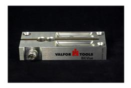
With its two holes of  $\frac{1}{2}$ " and 12mm diameter the Bit Vise will accept all commonly sized router bits, either directly or with the help of an appropriately sized collet sleeve (use a reducer bushing with an outside diameter of  $\frac{1}{2}$ " and inside diameter of  $\frac{1}{4}$ " for  $\frac{1}{4}$ " shanks, or  $\frac{1}{4}$ " shanks, or shanks).
